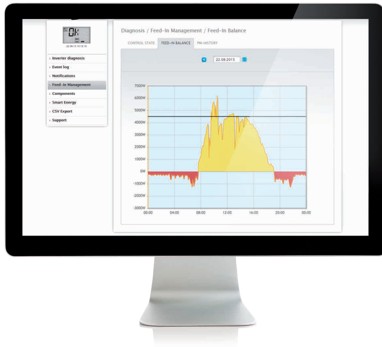
Feed-in management - feed balance: The times when there was a grid feed and when electricity was purchased from the grid can be seen at a glance in this graph. Negative values indicate that electricity was purchased from the grid and positive values that there was grid feed.
